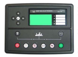
The use of Deep Sea DSE7320, DSE7220 or DSE6120 controllers is the control screen of the automation unit and the most basic configuration of unattended automation. The control panel is capable of receiving remote on/off unit control signals (ATS control).
